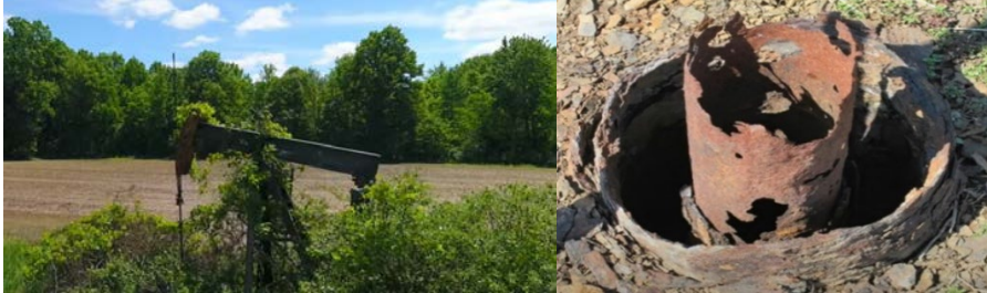
Orphan well in a field and, a well pipe visible on the ground
