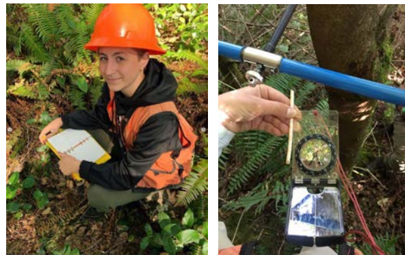
Coral uses an increment borer to extract a wood core sample and measures to determine tree growth, age, and general health on Confederated Tribe of Siletz Indians forested land
