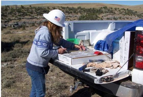
Solid Minerals Branch Geologist logging drill core, Crow Reservation, Montana
