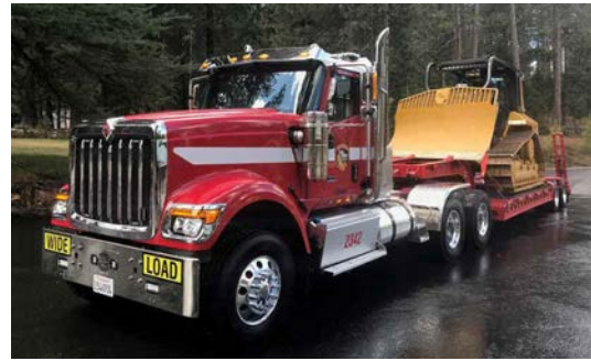
Fire dozer, transport tractor, and transport trailer
