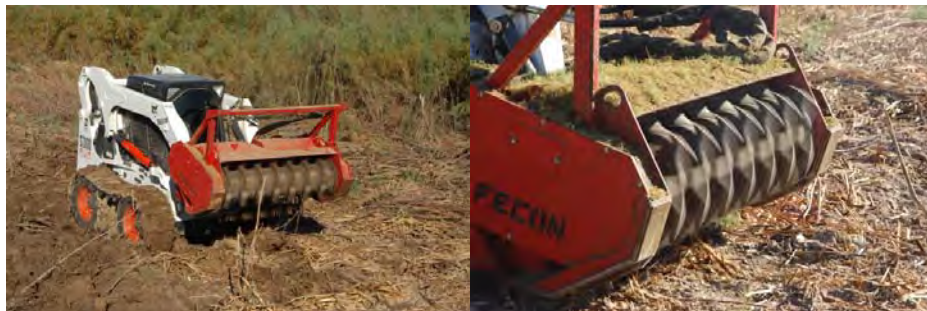
Figure 9-2. A Bobcat with a brush hog mower attachment removing invasive weed. Photo courtesy of Fred Phillips Consulting, LLC.
