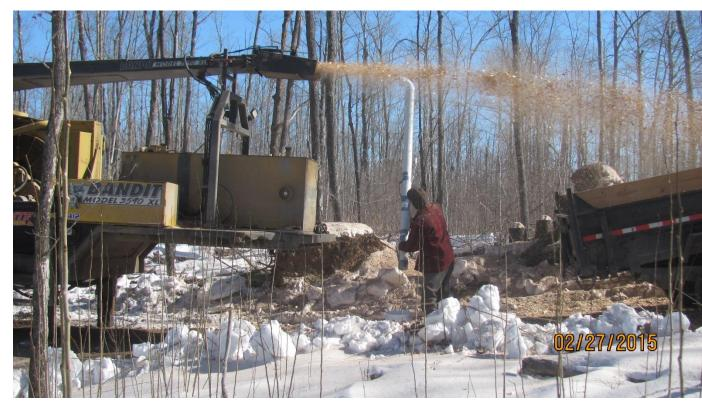
Final samples are collected from the operational chip stream to determine moisture, heat and ash content from the pile cross-section. Samples are collected during the chipping of the pile to compare drying effects within the residue piles.
