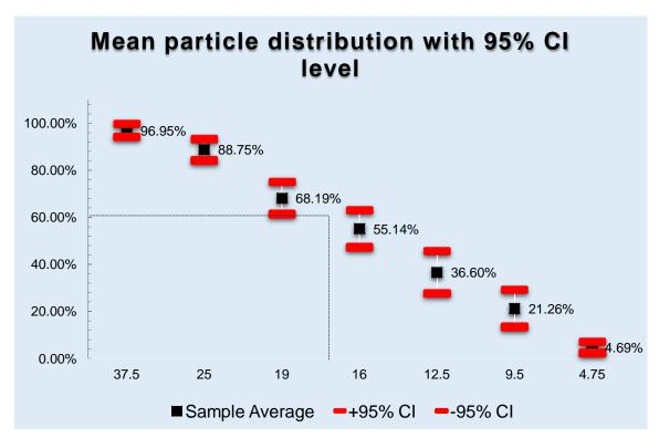
Particle size is displayed as the cumulative percentage that is passed through each successive screen size. Intersection shown above is the point where 60% percent of the material is passed by screens ( $P_{60}$ ).
