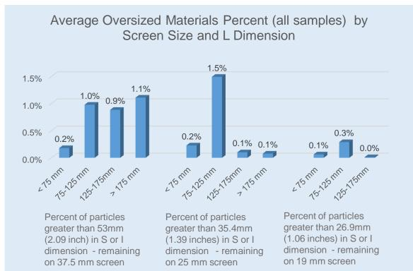
Oversize material is defined as the percentage of material, on a weight basis, that exceeds the cross sectional size of the screen in any axis (the particles L axis). Displayed by particles "L" length
