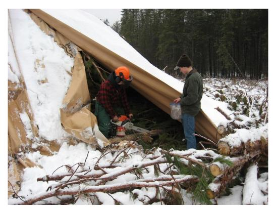
Initial and interim samples are extracted using a chainsaw and saw-dust collector. Each pile is sampled at butt, top and both sides. A total of 24 locations on each pile is extracted for assessment.
