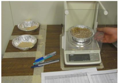
Each sample is oven dried using ASTM standards for woody biomass (ASTM D4442-07 & E871-82).
