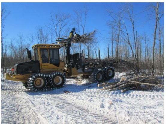
Harvest residue, comprised of tops and limbs is retrieved after processing the round wood. The tops and limbs are collected and piled to be dried in the field to enrich the recoverable energy.
