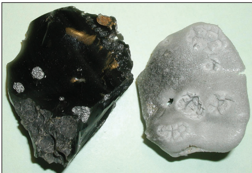
Figure 4-4 —On right: Extreme vesiculation in obsidian oven heated to 800 °C (1472 °F); sample also suffered severe weight and density loss. On left: Unheated obsidian from same source (samples courtesy of Anastasia Steffen).
