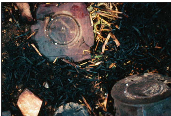
Figure 6-9 —Lead soldered cans in a test fire using straw as a fuel load. Note beads of melted solder.
