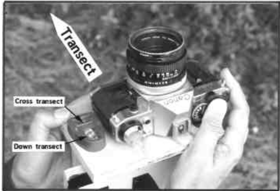
Figure 133—The camera leveling board is used to consistently rephotograph the tree canopy. Place the leveling board on top of the meter board for consistent height above the ground. Place the meter board at a right angle to the transect line. Move the meter board sideways to center the cross-transect bubble, then tilt the level board to center the downtransect bubble, and photograph.
