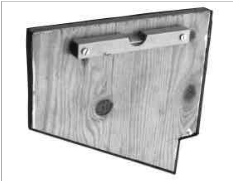
Figure 111—A line level is used to orient the board vertically. Obtain a 4- to 5-in-long line level and drill a hole in each end for a screw. Attach one end of the line level to the back of the meter board \frac{1}{2} in (1 cm) from the top. Then orient the board vertically by using a carpenter's level along one side. Hold the board in position, adjust the line level to horizontal, and carefully screw in the other end.
