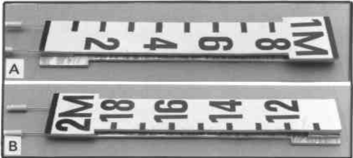
Figure 114—The 2-m board system. (A) Standard 1-m board with the top half folded underneath. (B) The folded board has been turned over to show the 2-m section.
