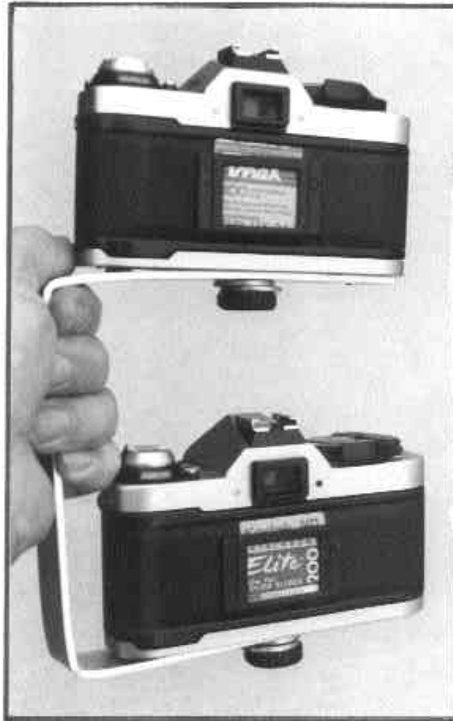
Figure 134—Double camera bracket for use when photographing in both color and black and white. The bracket is made from 1- by 1/8-in stock aluminum bar with holes drilled to mount the cameras. Identical cameras are recommended to simplify camera adjustment. Figures 135 and 136 illustrate construction details.
