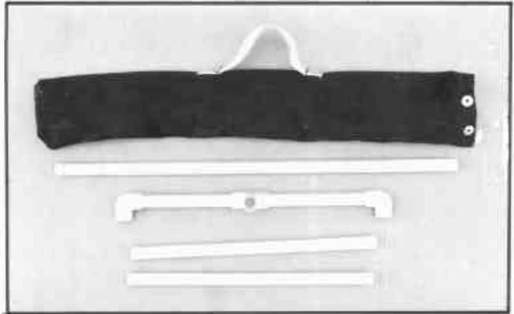
Figure 123—A1-ft 2 sampling frame disassembled with its carrying case. The case is made from canvas with a handle and two snaps at the open end.
