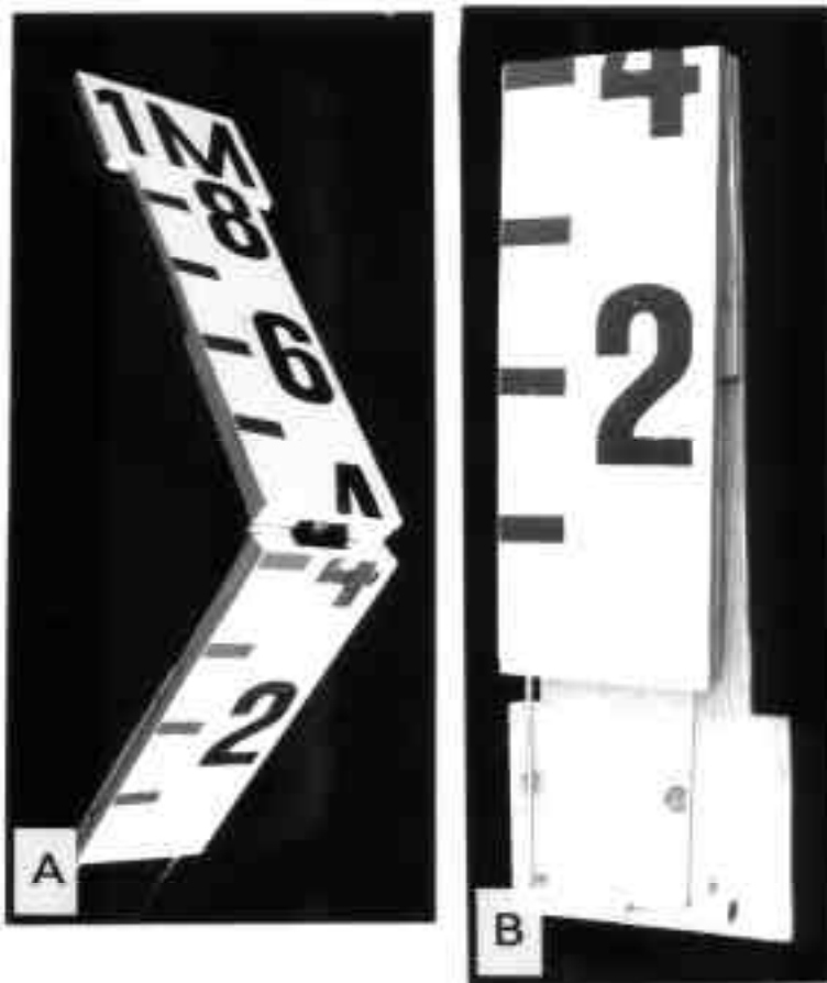
Figure 117—Folding 1-m board specifications. (A) Cut a standard 1-m board at 4 dm and install hinges and a barrel bolt. This offset is used to protect the spikes (B). Assemble the board before painting and application of decimeter marks to assure correct measurements.
