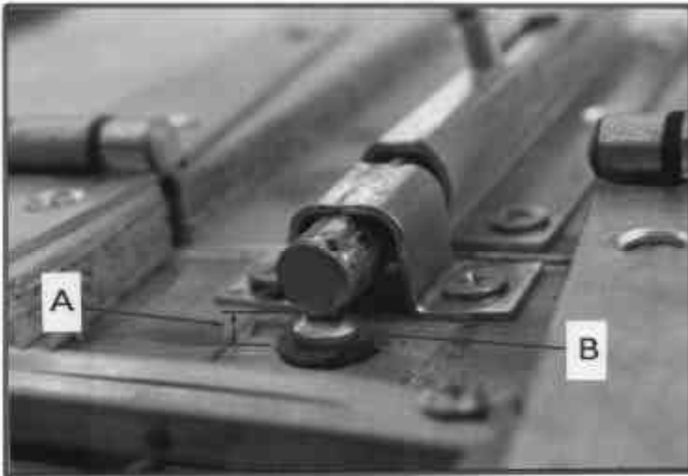
Figure 116—Adjusting screw and washer used to remove play between the barrel bolt and its strap, which will stiffen the two halves when unfolded. (A) Measure the distance between the bolt and the board. (B) Insert a round-headed sheet metal screw with enough washers to make the bolt fit firmly under the flange. Sheet metal screws are preferred because of their hardness. Pound the flange down if necessary.
