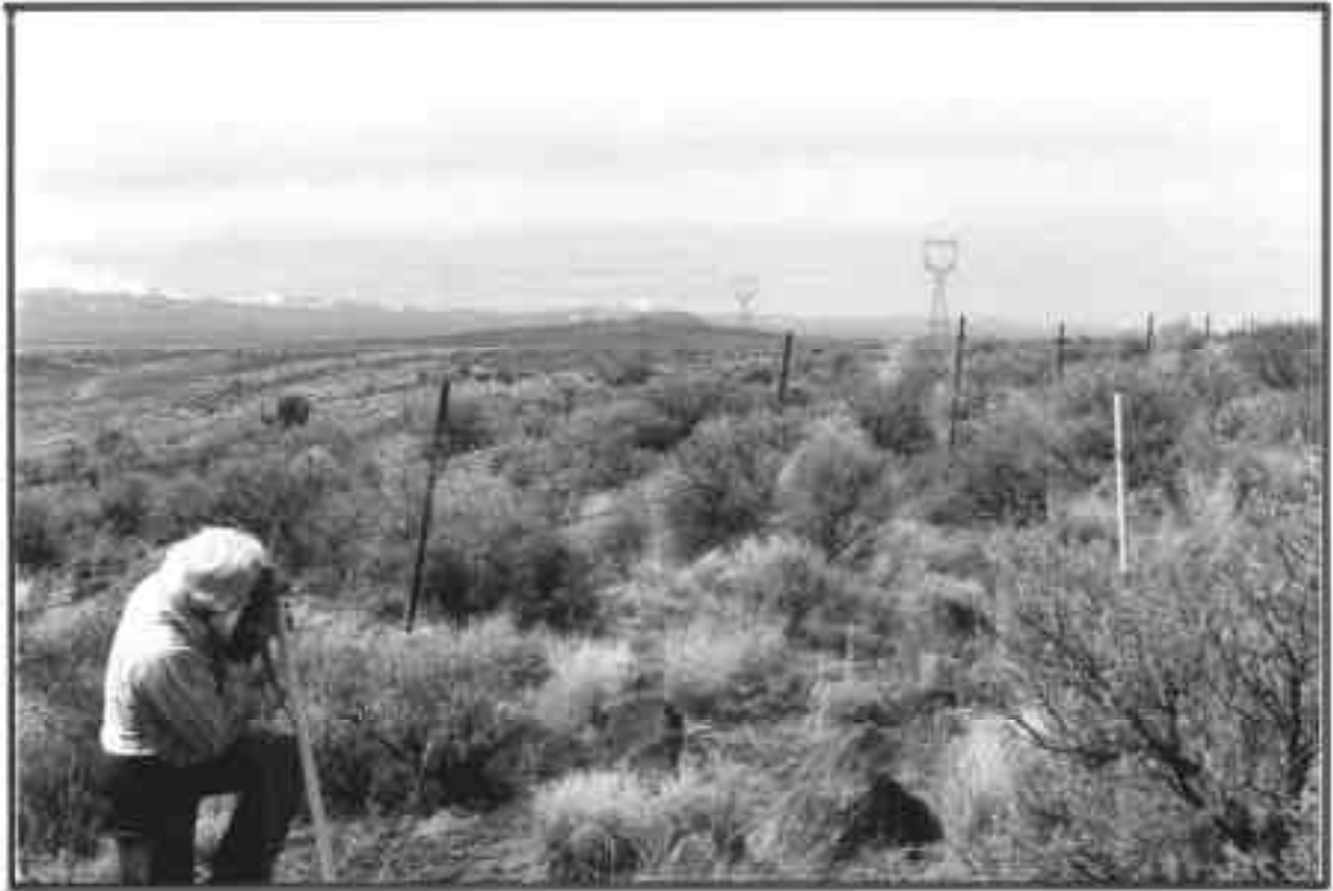
Figure 103—Technique for photographing the Robel pole. In this case, the camera is held in the “portrait” or vertical position. I prefer the “landscape” or horizontal camera orientation (see fig. 106) because it covers a broader area of ground at the Robel pole. Spikes on the bottom of the Robel pole and line pole (fig. 102) are 1/4-in steel rod 6 in long, which are capable of holding both poles upright.
