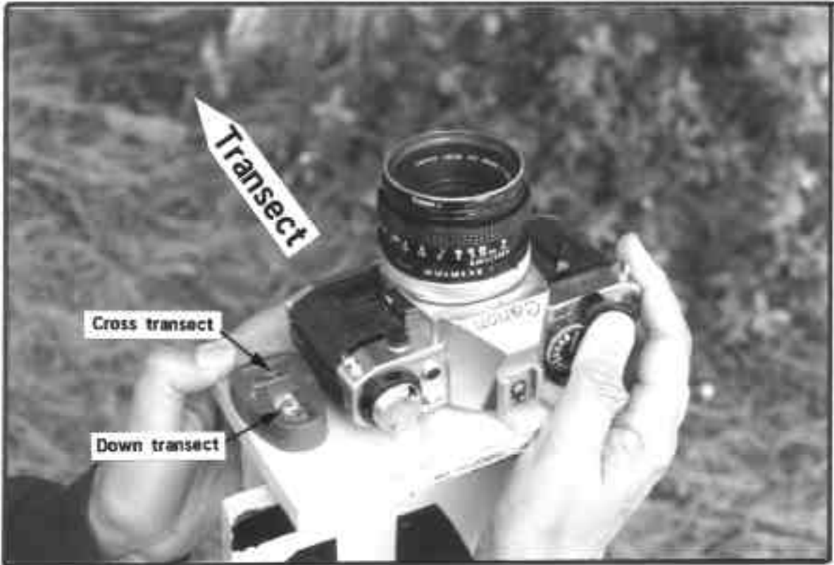
Figure 98—Tree canopy cover photography system. A meter board is placed crosswise (perpendicular) to the transect at foot marks 0, 25, 50, 75, and 100. Hold camera level board on top of the meter board and place the camera on the level board. First center the cross-transect level by moving the meter board sideways. Then tilt the camera level board so the down-transect-level is centered, move your head out of the camera view, and photograph.
