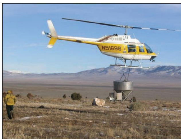
Figure 14-3 —Aerial seeding operation as part of the Emergency Stabilization Plan following the 2004 Chrome fire in southern Nevada. (BLM, Ely Field Office file photo.)
