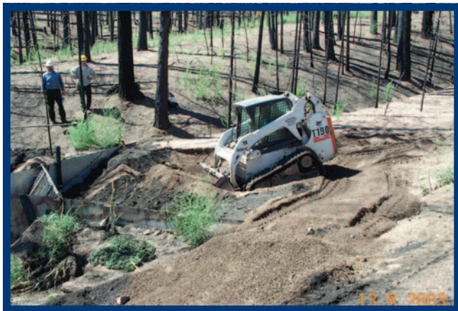
Figure 10.4 —During a short duration high intensity rain event, this research sediment trap was filled. Using pre- and postsurveys, Hydrologist Bob Brown and Engineer Joe Wagenbrenner measure the sediment collected with the help of a skid-steer loader. Research plots are in high severity burned areas of the 2002 Hayman Fire, Pike-San Isabel National Forest near Deckers, CO. (Photo by J.Yost).
