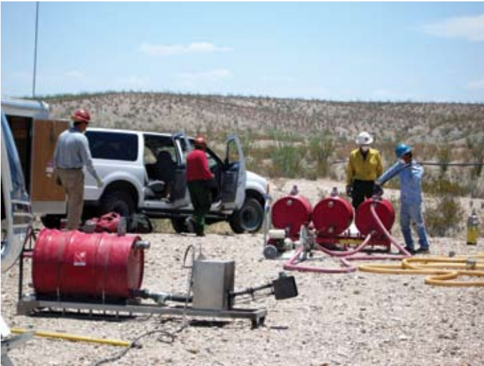
Helitorch and modular mixing system Big Bend National Park
