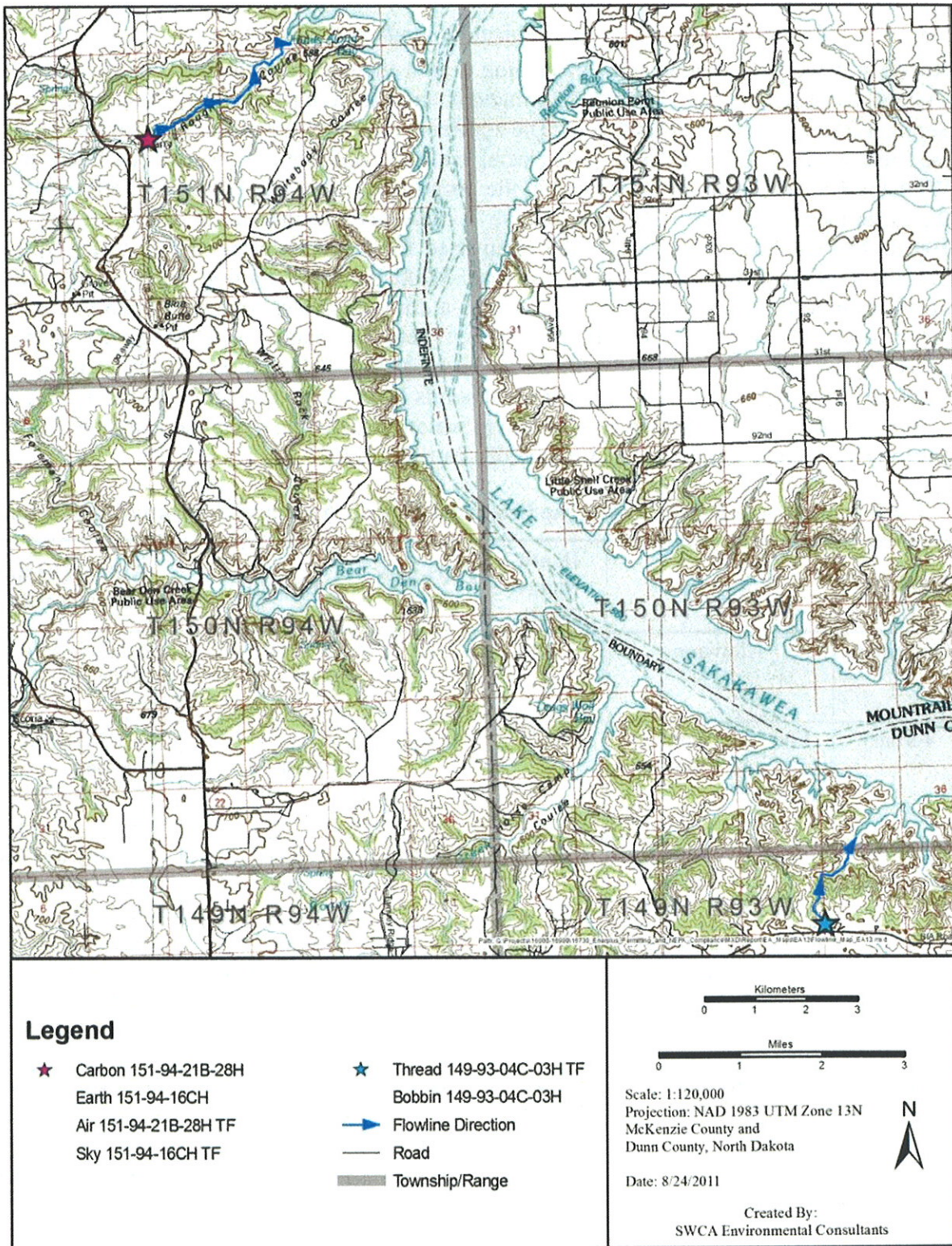
Figure 3.4. Surface runoff and drainage direction from each of the proposed well pads (North Dakota Department of Health, Division of Water Quality 2010).
