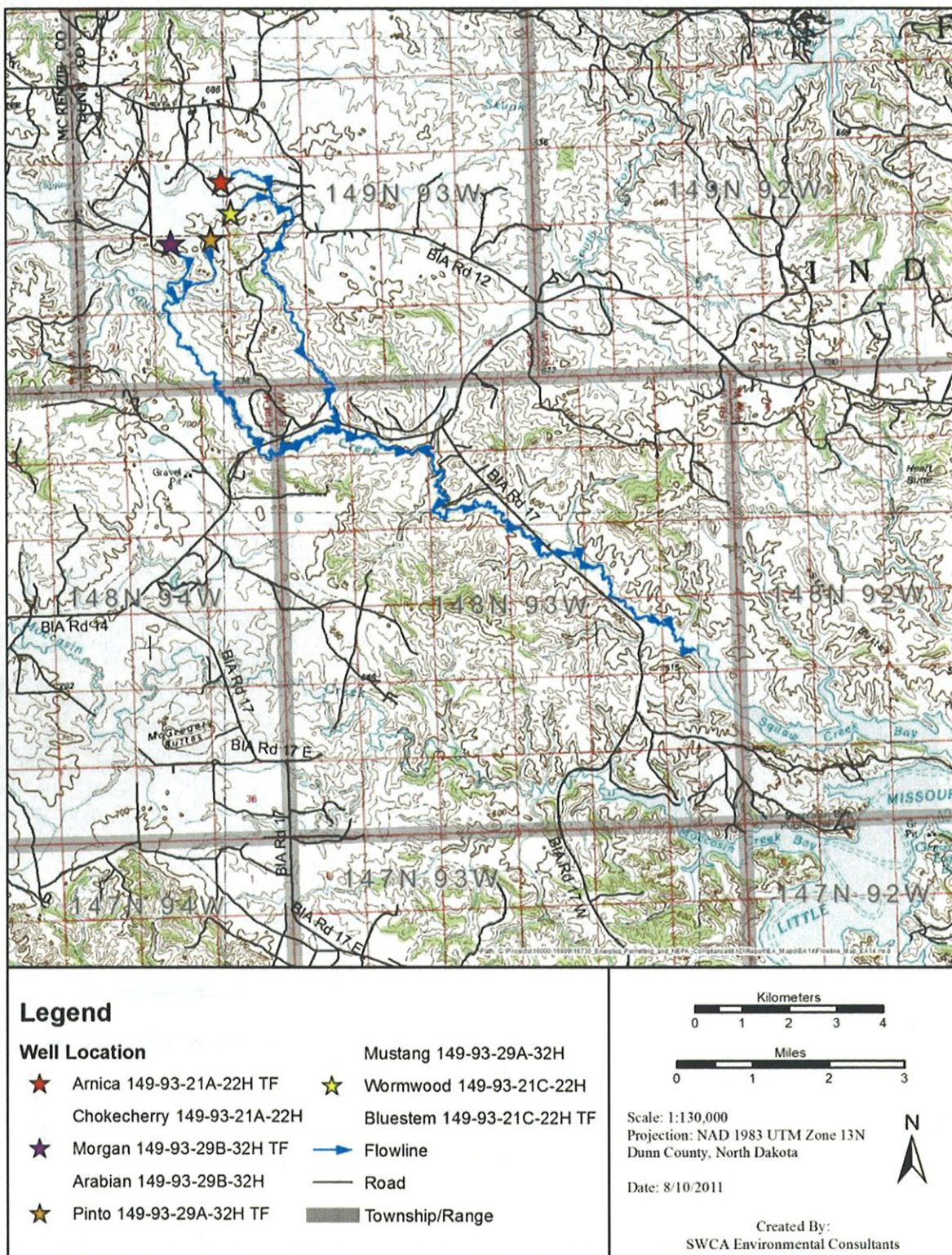
Figure 3.4. Surface runoff and drainage direction from each of the proposed well pads (North Dakota Department of Health, Division of Water Quality 2010).
