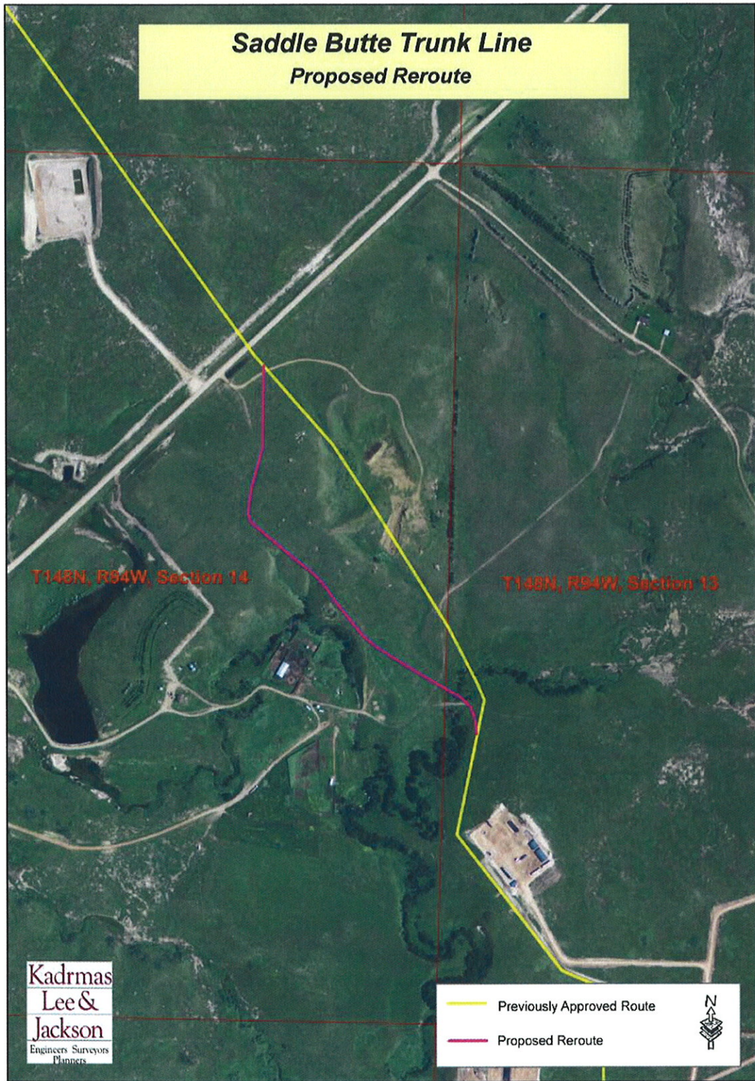
Figure 3. Saddle Butte Pipeline Reroute
