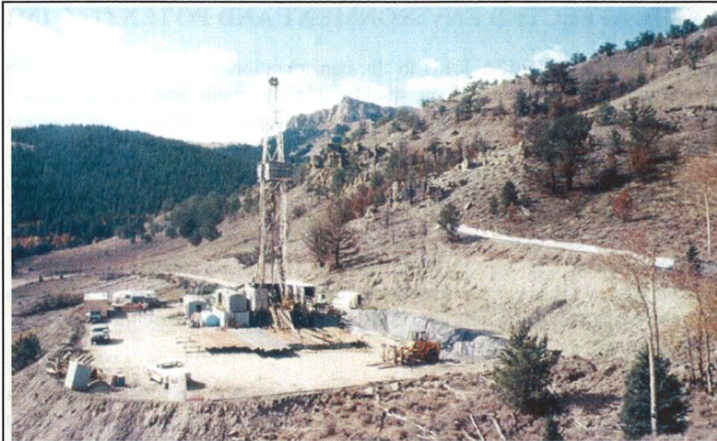
The well pad and access road are constructed to the minimum size necessary to safely conduct drilling and completion operations.
