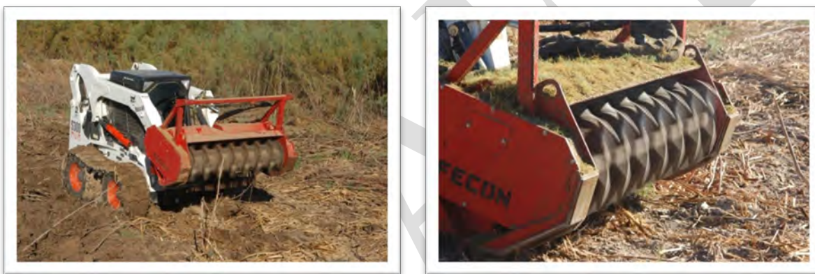
Figure 9-2. A Bobcat with a brush hog mower attachment removing noxious weeds. Photo courtesy of Fred Phillips Consulting, LLC.
