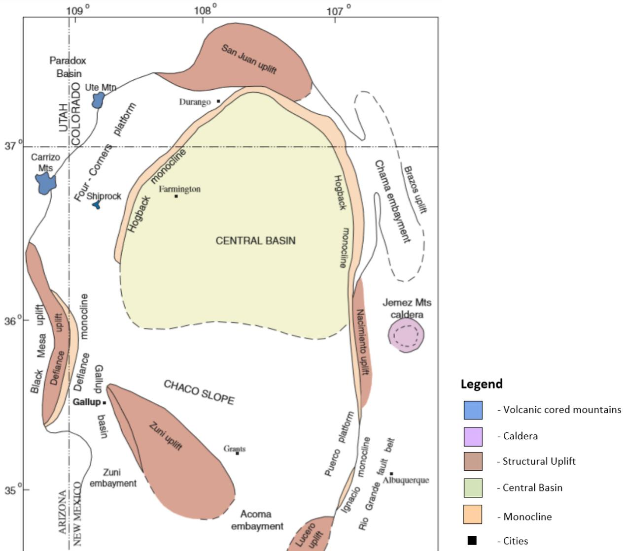
Figure 3. Index map showing the geographic and structural elements of the San Juan Basin (Fasset, 2010). Areas of steeper dip(monoclines) are patterned; arrows indicate the direction of dip. The dashed line separating the central basin from the Chaco slope is drawn approximately along the outcrop of the Pictured Cliffs Sandstone.
