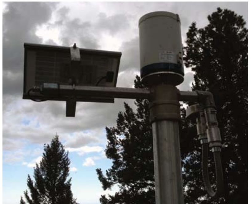
Peralta Ridge early warning system precipitation gage - tipping bucket. ~ Photo by Weiss, 2013
