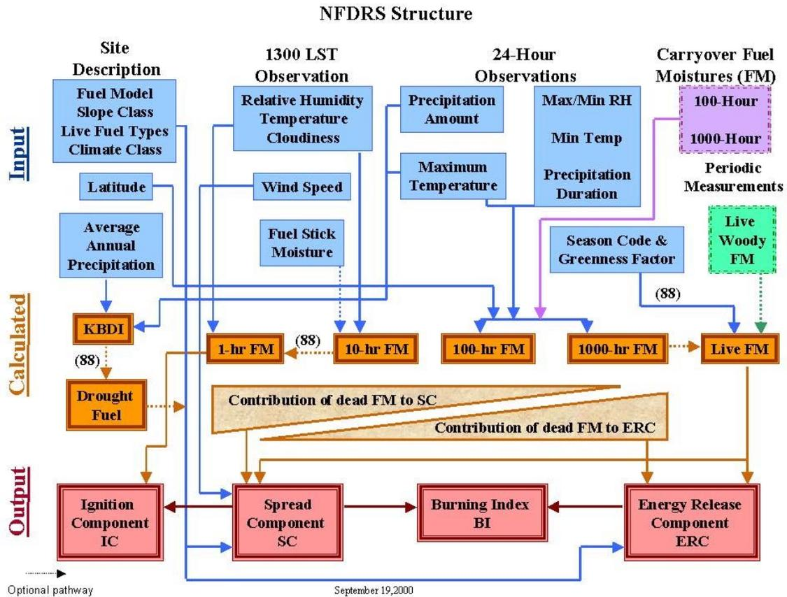
**2.0.2 Figure 2 - Flow of Information In and Around the NFDRS Processor**
