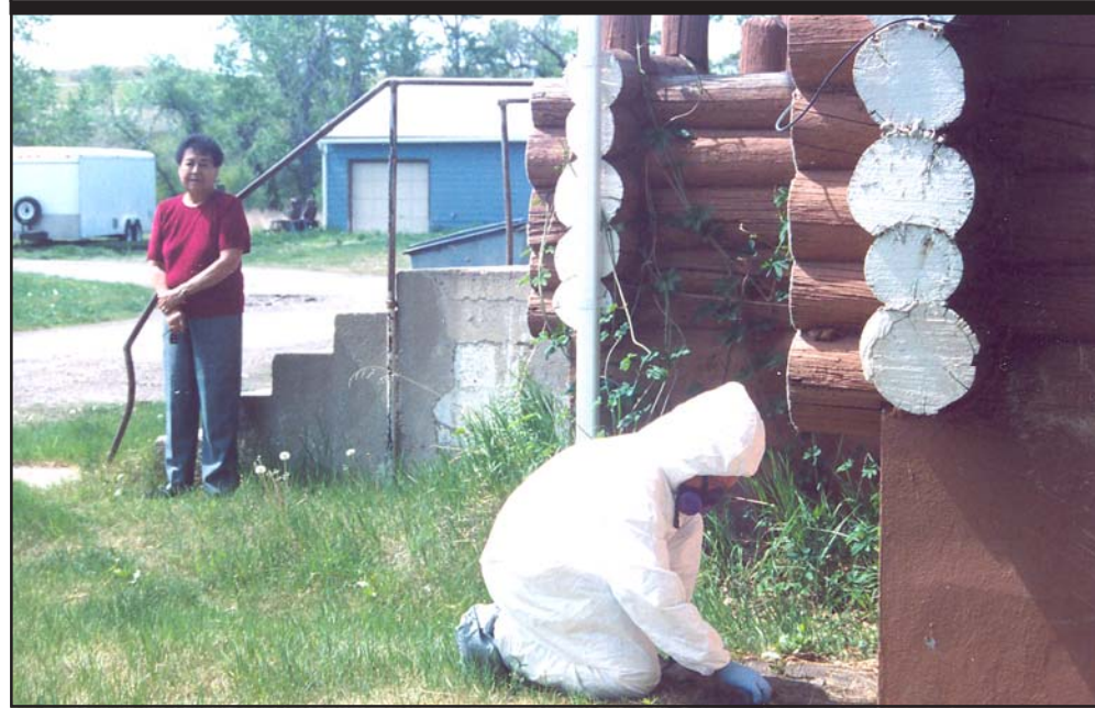
Darlene Parker, a Business Tech at the Blackfeet Dormitory, watches Industrial Hygiene Technician Matthew Olson test lead contamination levels near the foundation of her log home on dormitory grounds.
